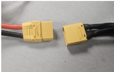
Figure 50: LiPo Connectors for the Battery Wires (Pictured Left) and Power Wires (Pictured Right)
